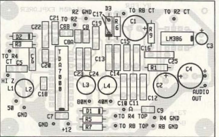
Figure 5. PC board parts placement.
